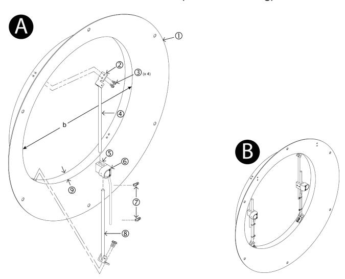
Step 1. Select a location on the fan that allows clearance for probe placement and installation.
