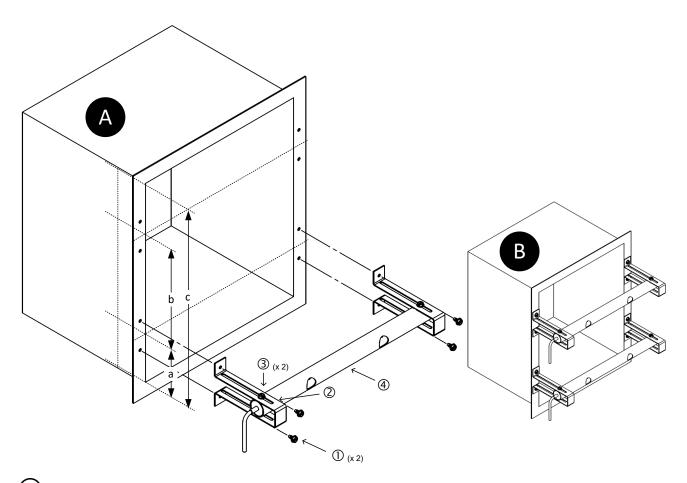
Standoff probes may be mounted immediately upstream of an outdoor air intake damper in applications where placement limitations prevent the installation of an extension sleeve before the damper.
