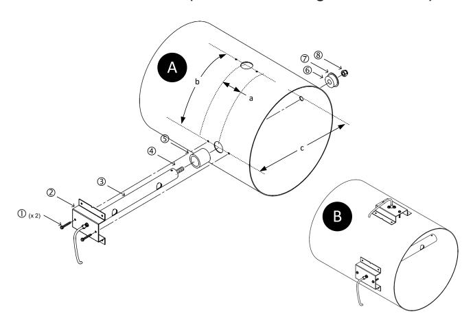
Step 1. Select a location in the duct or plenum opening that meets or exceeds EBTRON's recommended placement guidelines.
